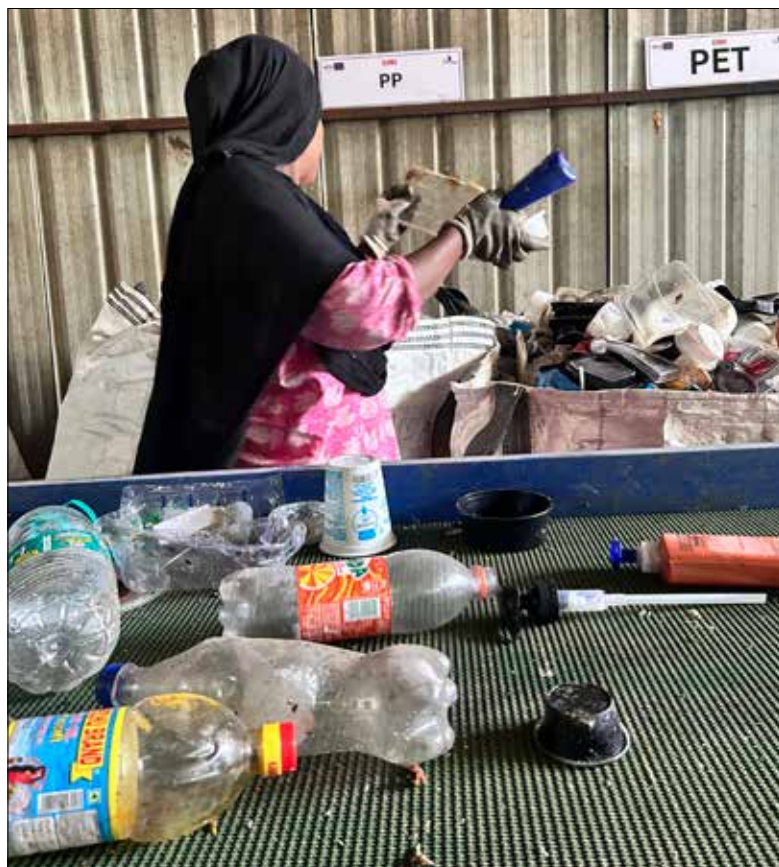
Figure 11 : Dry waste sorting by a woman waste worker using Conveyor belt at Sushant Lok DWCC
