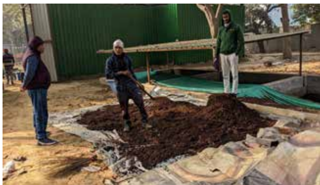
Figure 7 : Curing of compost at a community composting unit in ward 32
